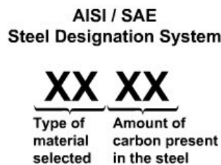
Figure 1: Schematic Representation of AISI/SAE Steel Designation System
